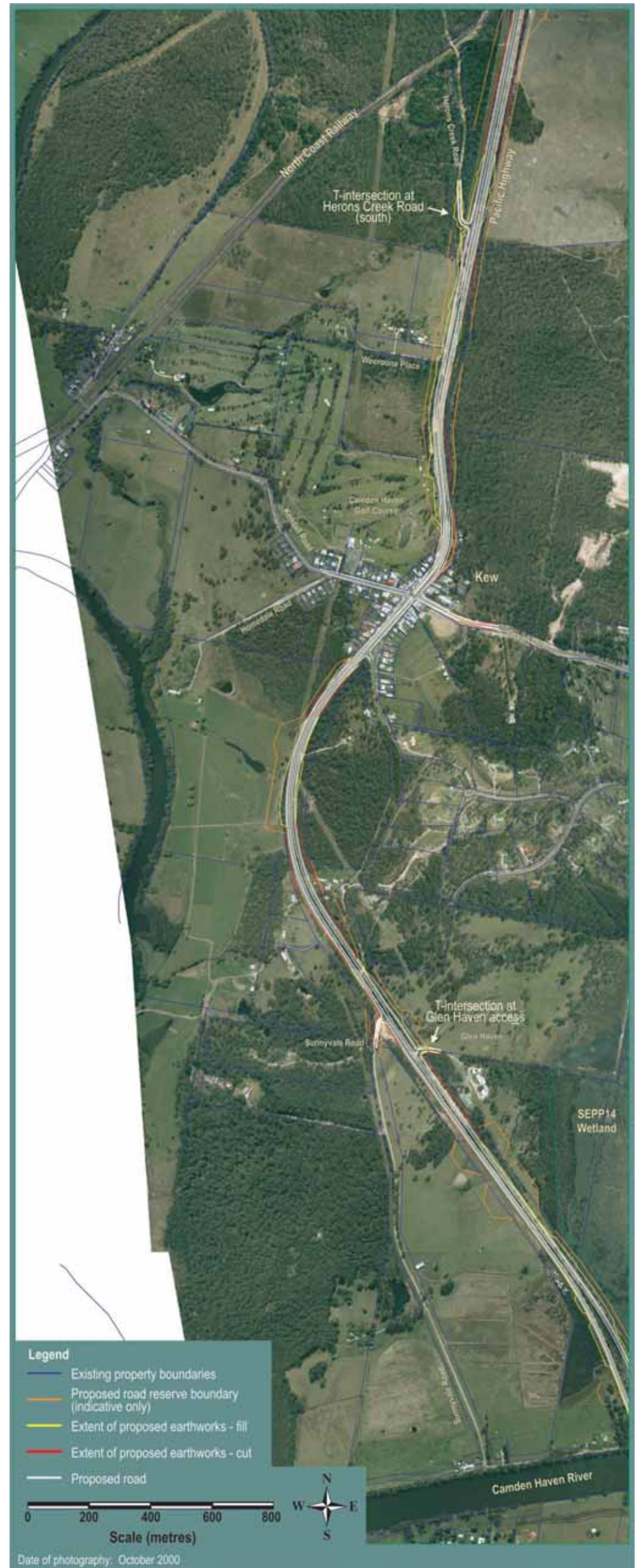
Figure 5-4D Route option K-D - Kew - Existing highway upgrade
