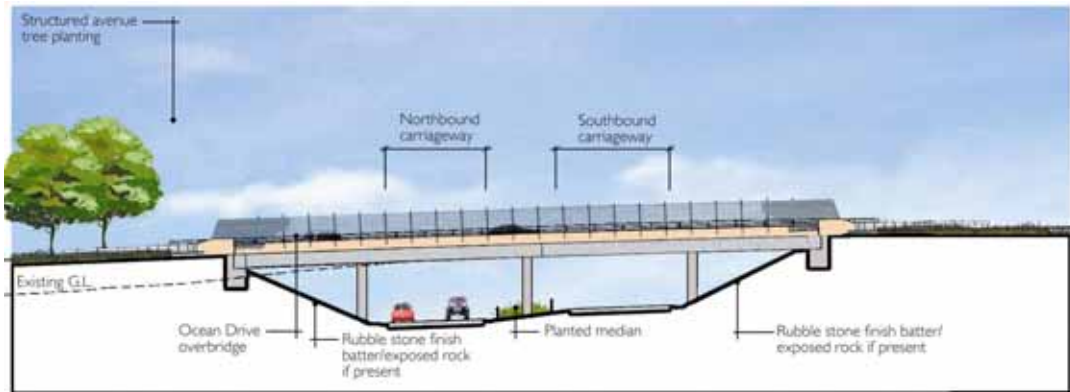
Figure 13-12 Ocean Drive overbridge – general arrangement looking northwards
