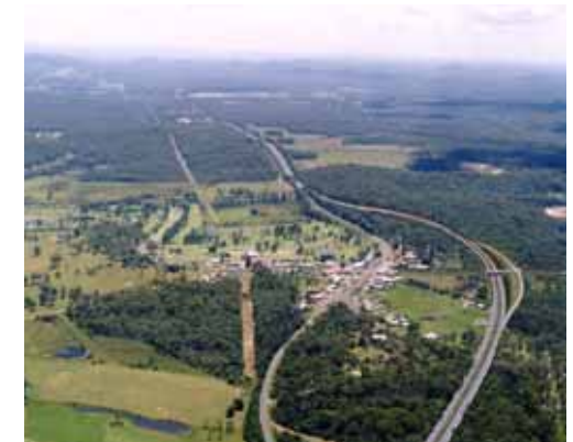
Photomontage of Kew looking northwards towards Herons Creek showing proposed Pacific Highway bypass and overpass
