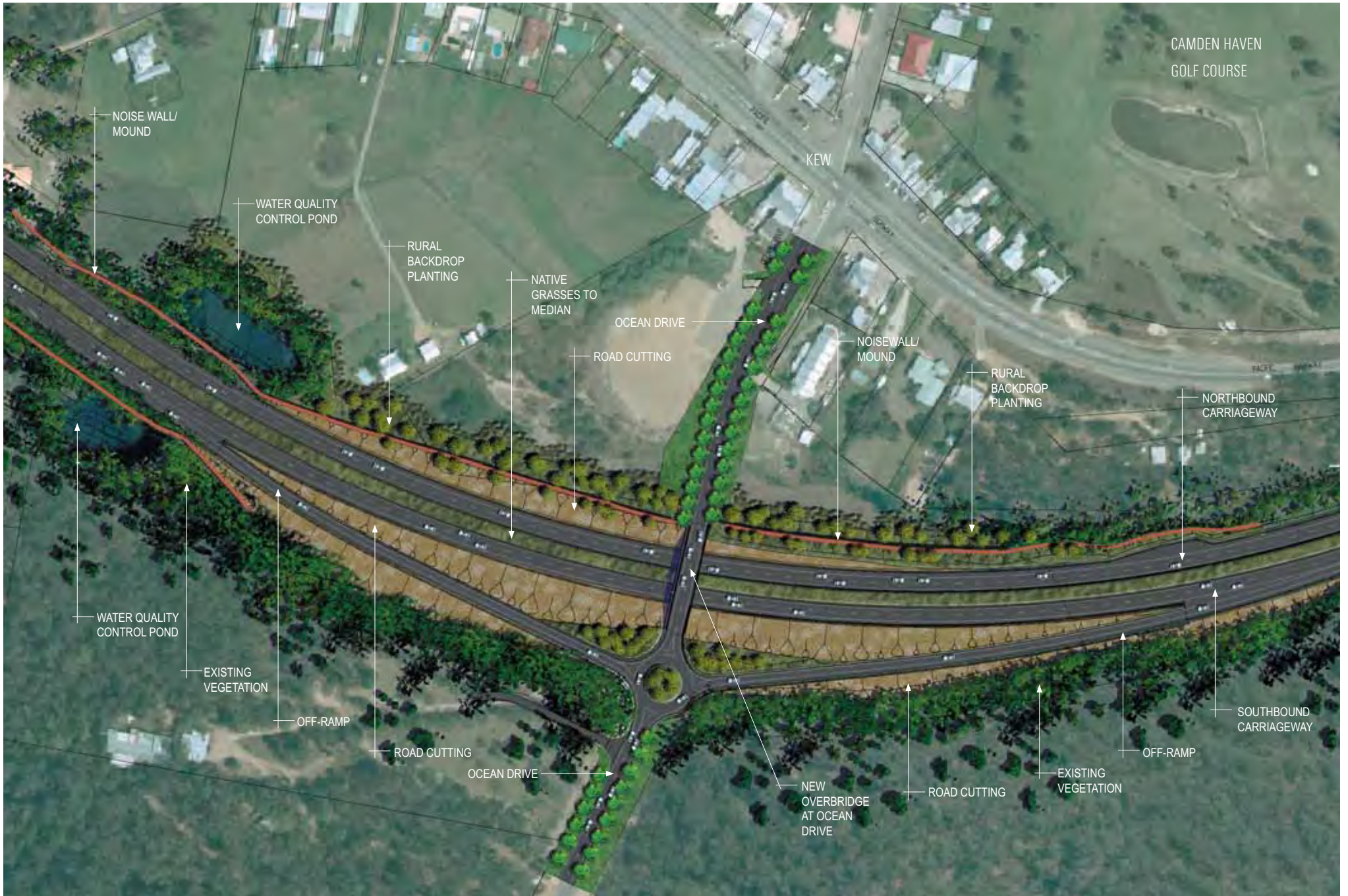
SCALE 1:2,000 PLAN P - KEW INTERCHANGE - DETAIL PLAN
